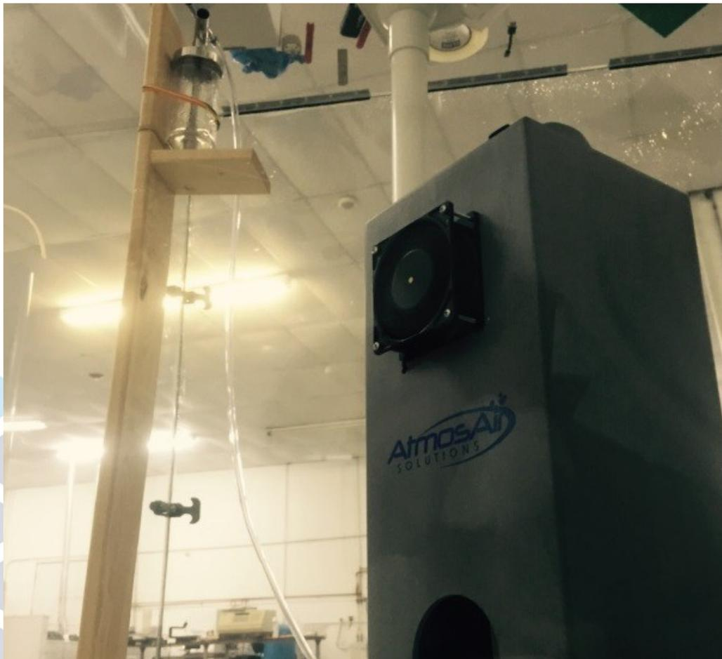
*Pictured Above: AtmosAir Matterhorn activated during treatment of air after aerosolization of microorganisms via Collison 6-Jet Nebulizer (Top Left). Testing configuration is such that the built-in fan (inflow) of the device is positioned near the point source of aerosolization and exhaust vent serves to re-suspend bioaerosols after treatment.*
